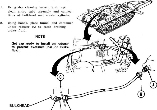
3. Using 13/16 inch wrench to hold reducer (A), use 11/16 inch wrench to remove tube connecting nut (B). Cap reducer (A).
