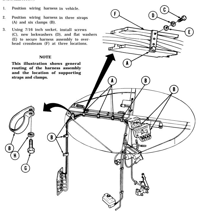
4. Using 7/16 inch socket, install screws (G) and new lockwashers (H) to secure harness assembly at six locations.
