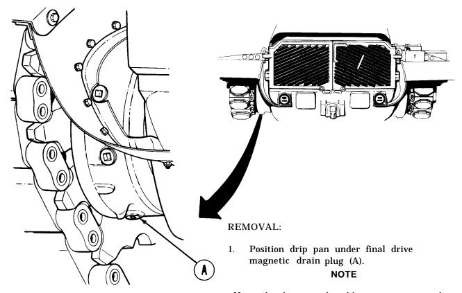
2. Using allen wrench or drive handle, remove magnetic plug (A) from final drive.
