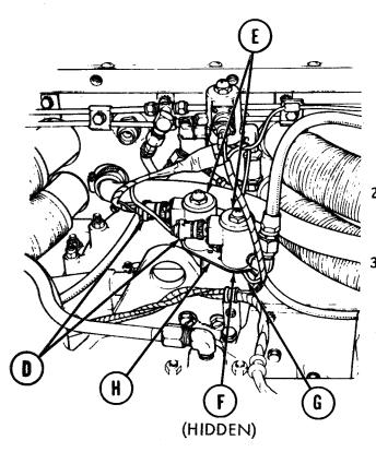
4. Feed female connector cables between exhaust manifold (J) and engine.
