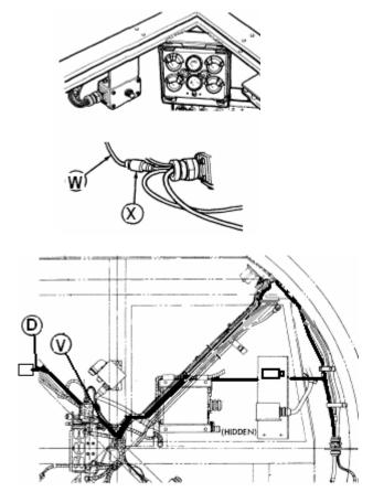
3. Route main power wiring harness (D) (CKT 49) from right side of vehicle to slave receptacle (U) located in front of driver.
