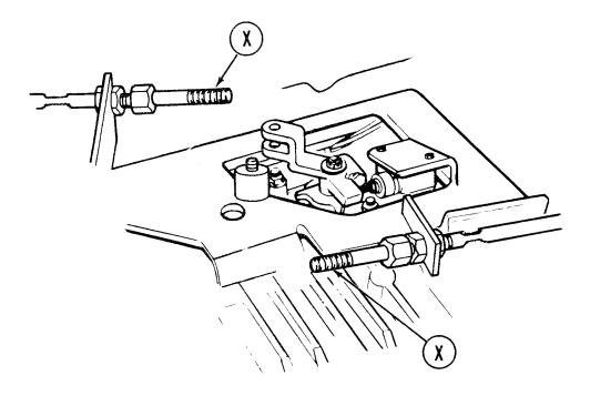
22. Install both clevises (Z) on rod ends. Thread clevis up to measured mark.
