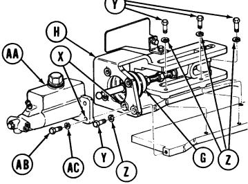
Remove web straps or ropes used to secure master cylinder.
