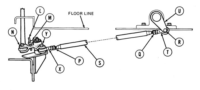
FORWARD INBOARD LINK ASSEMBLY
