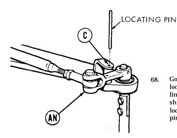
68. Go to right rear of vehicle and try to insert locating pin into alinement hole (C) and through link (AN). If locating pin can be inserted, shift linkage is in adjustment. Remove locating pin and go to step 126. If locating pin can not be inserted, go to step 69.
