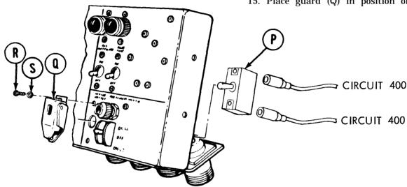
16. Using screwdriver, install two screws (R) and lockwashers (S) securing guard (Q) and heater master switch (P) to panel.
