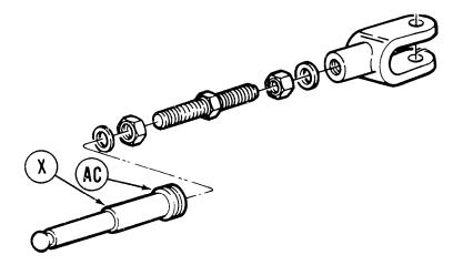
3. Inspect all parts for damage or excessive wear. Replace if unserviceable.
