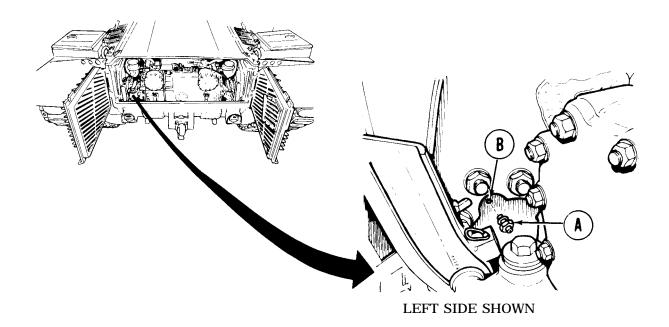
2. Inspect air pressure valve to make sure that vent cap is free to move on valve. Replace as required.
