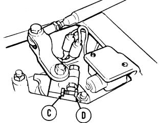
Using two wrenches, loosen jamnut (C) while holding screw (D).
