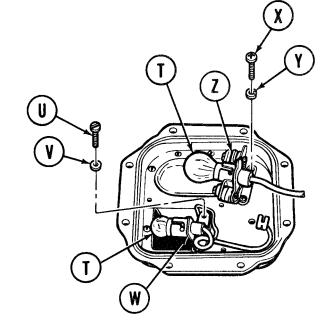
15. Using cross-tip screwdriver, remove two screws (X), and lockwashers (Y), holding the lampholder (Z) in place.
