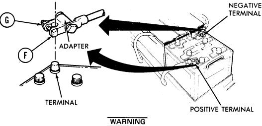
Do not let wrench handle touch hull metal while removing negative battery adapter. Arcing could occur and personnel could be burned.
