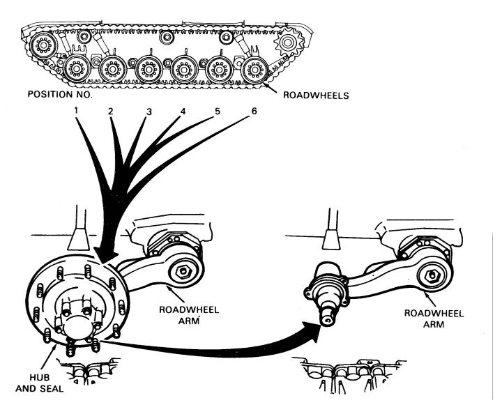
ROADWHEEL ARM (WITH HUB AND SEAL)
