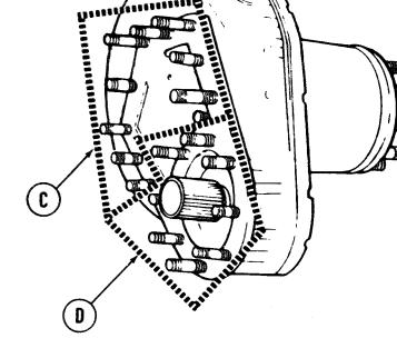
3. Thread two hex nuts on new stud and jam the nuts. Using 1-1/2 inch wrench on top nut, install new stud (B).
