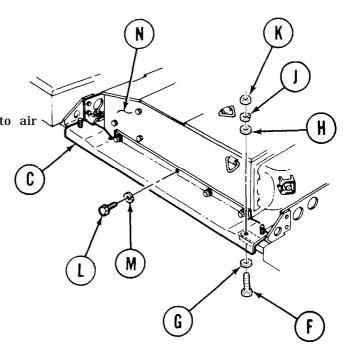
4. Remove fender extension (C) by lifting it up and away from vehicle.
