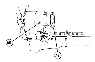
13. Remove gasket (AE) from starter drive adapter (AD). Throw away gasket.
