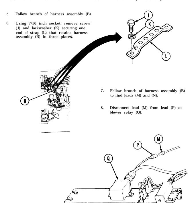
9. Disconnect lead (N) from heater feed circuit breaker (R).
