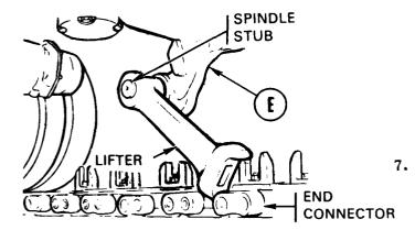
Using mallet, tap roadwheel arm lifter off spindle stub. Remove lifter.
