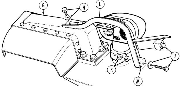
7. Using 1-inch socket, remove four screws and lockwashers (N) holding fender support No. 1 (G) to hull (M).
