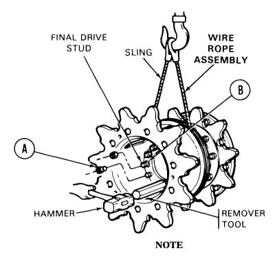
These vehicles may use either one piece nut and bushing assemblies or two piece nuts and bushings to secure sprocket and hub assembly to final drive. If one piece do steps 6, 7, and 11. If two piece do all steps.
