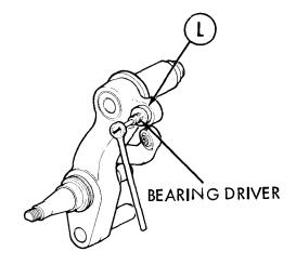
11. Secure bearing tool assembly: to bearing (L) with screw and nut, Install puller to bearing tool assembly and remove bearing (L). Discard bearing (L).
