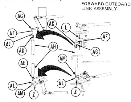
49. Using 9/16 inch wrench, adjust shifting rod bearing end (AG) clockwise until shifting rod (AH) is past hole (AJ).
