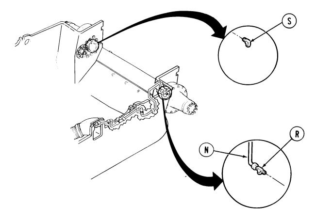
19. Using adjustable wrench, install elbow (S) into right final drive.
