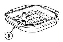
19. Remove blue lens (AC), and gasket (AD) by pushing up from outside of door (B).
