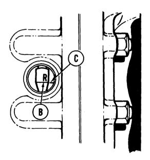
3. Check whether index line (B) marked R and index mark (C) are lined up.
