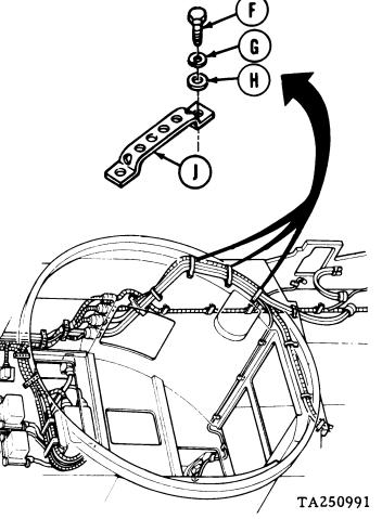
3. From engine compartment, using 7/16 inch wrench, remove screws (F), lockwashers (G), and flat washers (H) from three straps (J)
