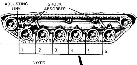
There are six support housings on each side of vehicle. The procedures for all six are identical except that no. 1 housing is not interchangeable.
