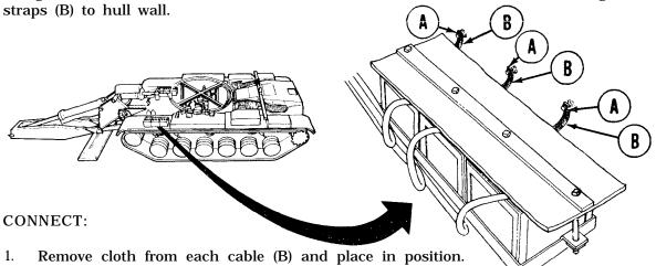
1. Remove cloth from each cable (b) and place in position.
