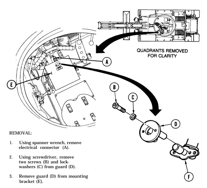
4. Remove selector switch (F) from mounting bracket (E).
