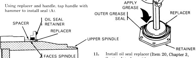
Section I) to face with spacer on upper spindle of arm.
