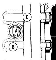
16. Fully apply brakes (TM 5-5420-202-10). If index line (B) marked A moves past index mark (C), brake is too loose.
