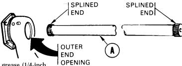
2. Fill outer end opening with grease (1/4-inch deep).
