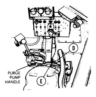
2. Disconnect two connector leads (D) and (E) from manifold preheat switch on purge pump handle.
