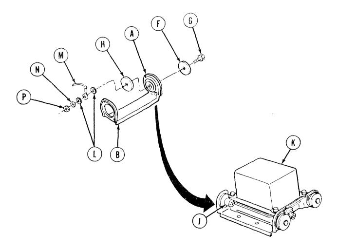
10. Using steps 6 through 9, except omitting lockwasher (L) and ground strap (M), install power supply (K) onto two brackets (B).
