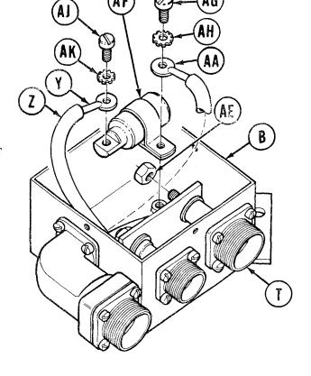
24. Using screwdriver, install screw (AJ) and lockwasher (AK) securing terminal (Y) to capacitor (AF).
