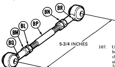
Using vise and 9/16 inch wrench, turn rod bearing end (BM) clockwise or counter-clockwise until distance between centers of rod bearing ends (BM) and (BN) measures 5-3/4 inches.
