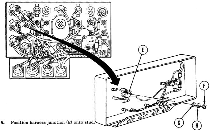
6. Using socket, install nut (F), flatwasher (G), and lockwasher (H) securing harness junction (E) to panel.
