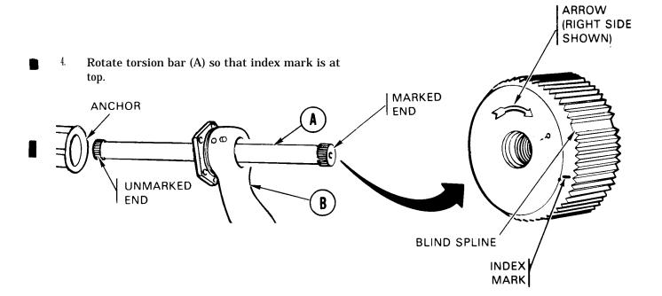
5. Push bar (A) through housing until inside end enters anchor on other side of vehicle. When this is done, about 1/2 inch of bar will be out of housing.
