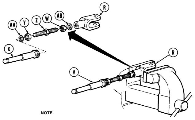
Clevis (R) and nut (W) have left hand threads. Push rod (X) and nut (Y) have right hand threads.
