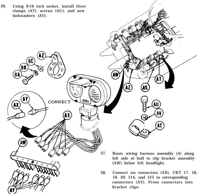
Using socket, install two straps (AZ), screws (BA), new lockwashers (BB), and flat washers (BC).
