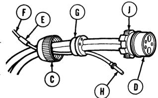
6. Pull lead assembly (F) back through bushing (G) and retaining nut (C).
