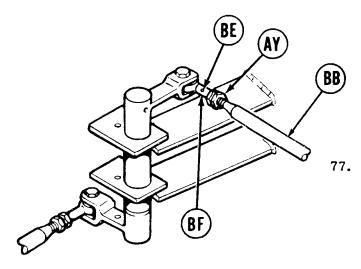
Using small diameter wire, check to see if shifting rod (BB) is past holes (BD) and (BE). If shifting rod (BB) is past holes (BD) and (BE), do steps 78 thru 80. If shifting rod (BB) is not past hole (BD), do steps 82 thru 91. If shifting rod (BB) is not past hole (BE), go on to step 92.
